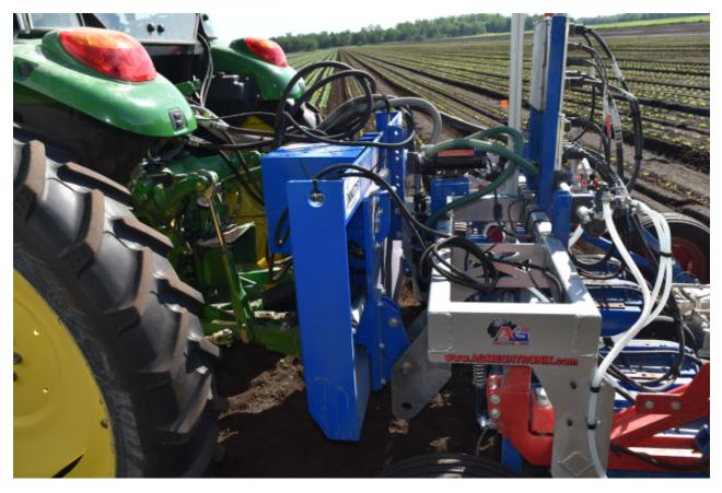
The Innotag sliding quick hitch incorporates the latest technology to make row crop cultivation both fast and accurate. Robust construction and high capacity cylinders give it the ability to handle the heaviest 3 point'mounted cultivators. When combined with the Innotag Culticam, you can cultivate as soon as rows are visible.
