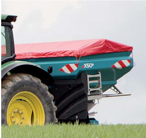
Mud guard protectors in imperishable composite material (as standard) and supple extensions (option): total protection against projections of earth during high speed spreading in wet conditions and easier cleaning
