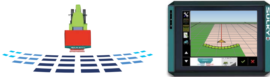
In ISOBUS ECONOV controls 12 equal sections whatever the working width (here in full width with the 12 sections open)
