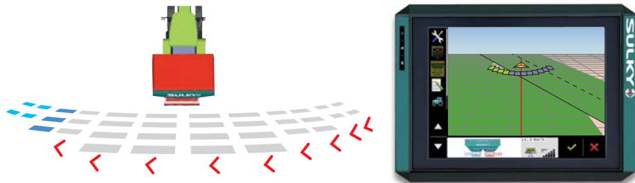
Right-hand side closed, progressive closing of the left-hand sections, from the centre to the outside
