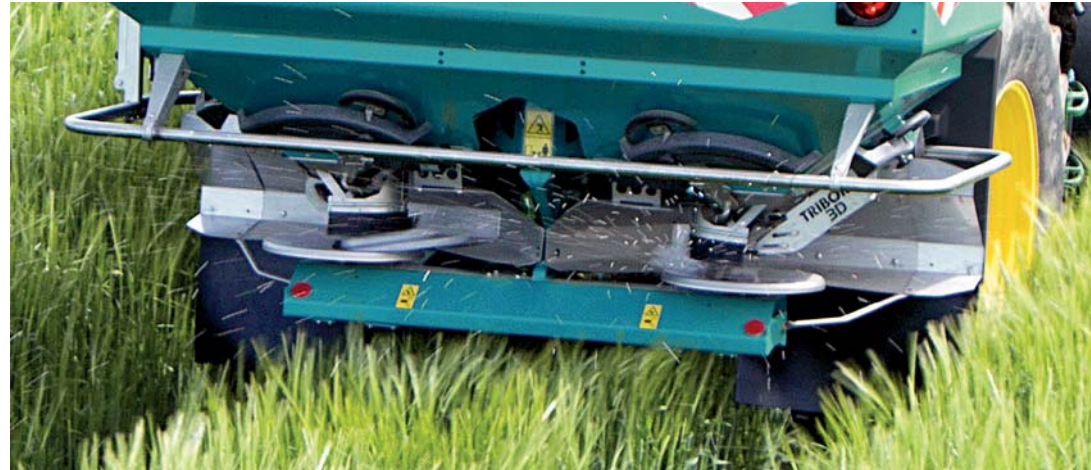
Highly resistant carbide-coated blades as standard on all the X50+ and the X40+ W weighing, X40+ Stop&Go and X40+ ECONOV versions
