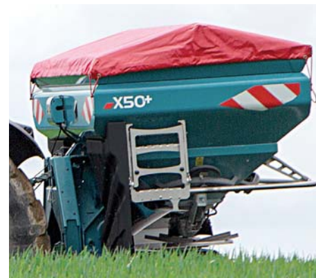
Hopper access ladder: - Placed on both left and right on X50+ (standard) - Placed on the rear left on X40+ (option)
