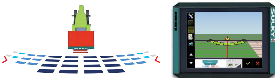
On arriving in a straight headland the sections close progressively from the outside to the inside, thus respecting the real shape of the spreading area... in a CURVE!
