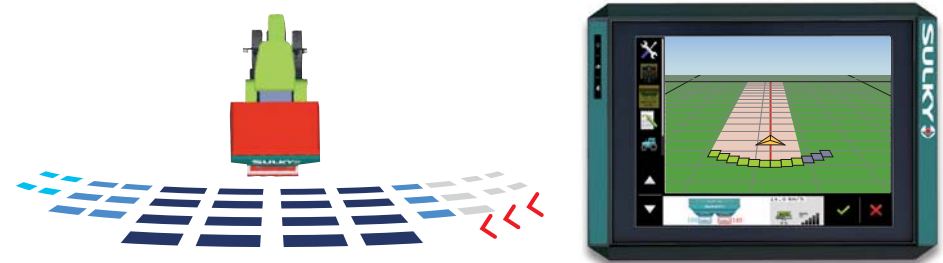
If the spreading width is reduced, during the last pass for example, the sections close automatically according to the width remaining to be spread (here 3 sections are closed on the right-hand side)
